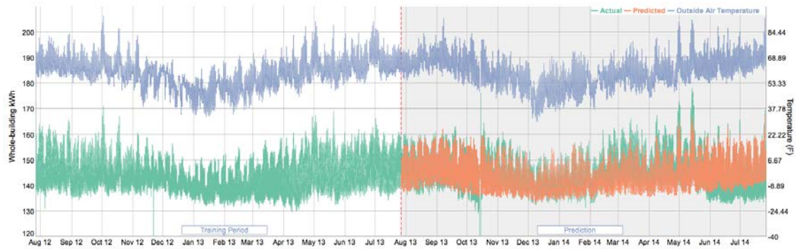
Figure 2. Actual and model-predicted energy data, overlaid with outside air temperature, for a 12-month training period and 12-month prediction period.
